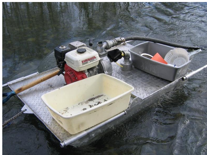
Figure 2. Hydraulic sampling equipment transported on raft.
