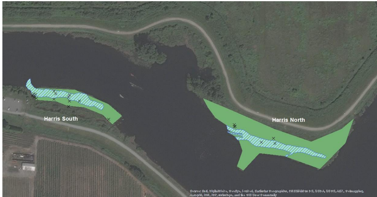
Figure 6. Final shape of excavations to create marsh habitat and locations of anchored wood at the Harris South and Harris North restoration sites.
