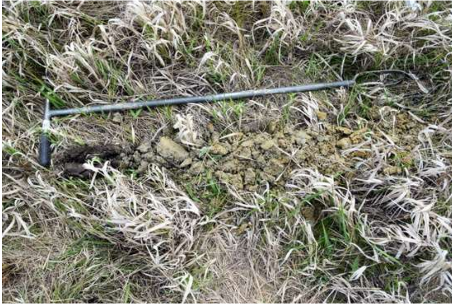
A soil auger was used to measure soil texture and to determine the elevation of groundwater at each wetland restoration site.
