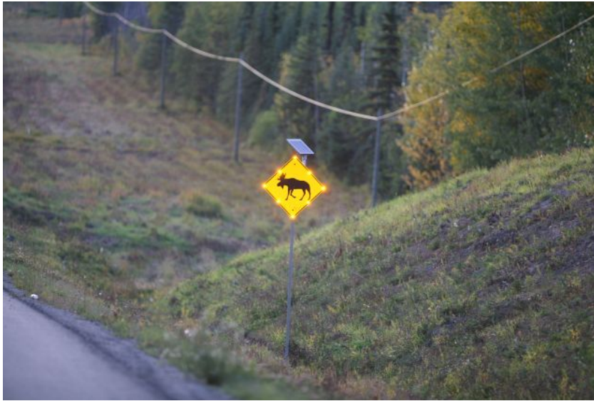
Figure 8. LED-enhanced moose collision warning sign, located near Tabor Mountain, Highway 16 east of Prince George (RV Rea).
