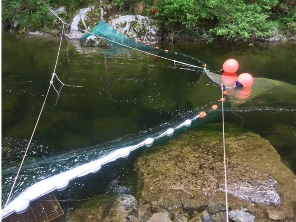
Figure 18. Fyke Net in Tailrace below the Discharge Tunnel (provided by LGL).
