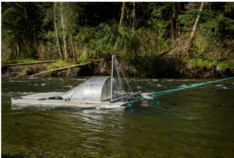
Figure 20. Photo of a Rotary Screw Trap.
