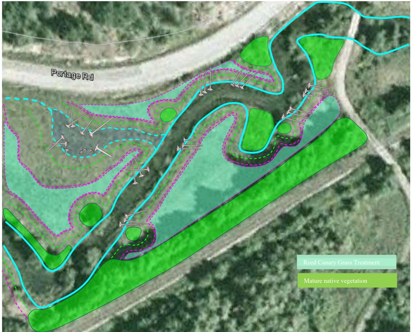
Figure 27. Overview of proposed restoration measures at 9523 Portage Road. Solid blue lines indicate Gates Creek Top of Bank (TOB). Dashed blue line indicates proposed off-channel habitat. Dashed green line indicates approximate limit of vegetation stripping at TOB. Dashed purple line infilled with mint-green shading indicates approximate limit of reed canary grass treatment. Bright-green shading indicates area of mature native riparian vegetation to be retained.
