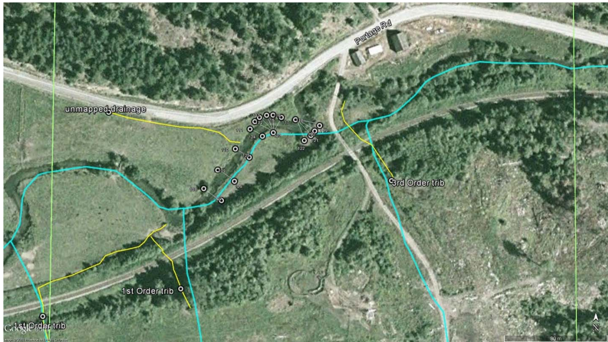
Figure 5. Overview of FWCP owned property at 9523 Portage Road. While lines indicate depth-velocity transects from October 2017. Blue lines indicate mapped drainages. Green lines indicate property boundaries, and yellow lines indicate observed drainage locations.
