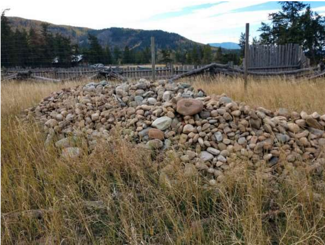
Photo 6: Huge piles of rock moved from hayfields were used to restore the creek bed. Having this material on-site saved money by not having to haul it in from an aggregate pit.
