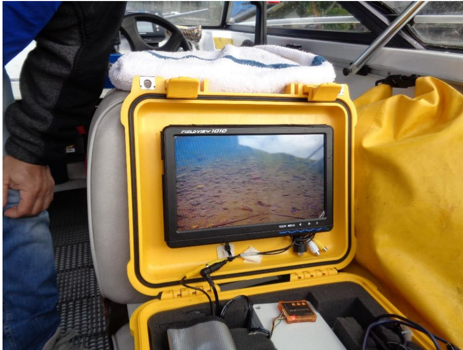
Photo 5. Video camera monitor for real time viewing of underwater transects.
