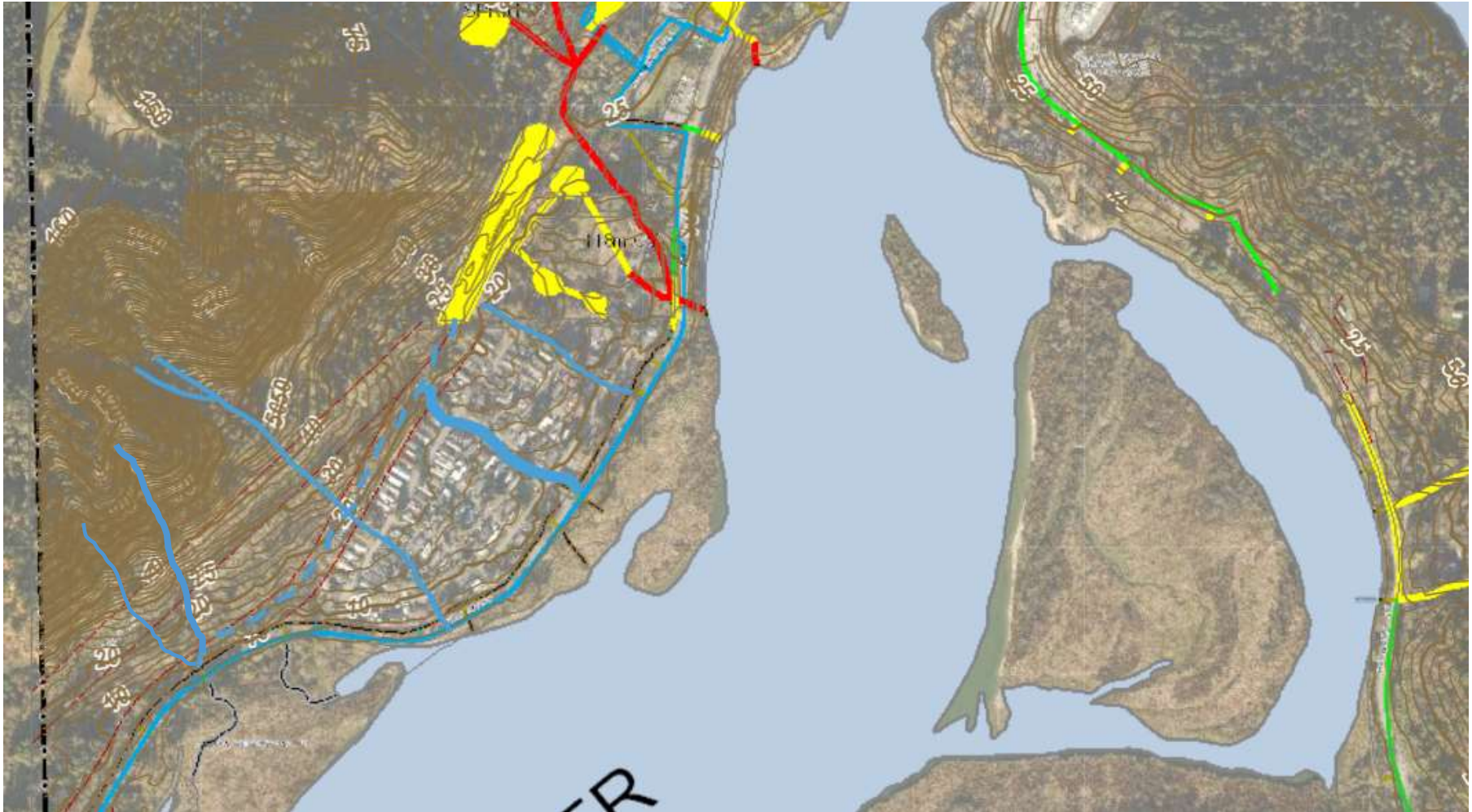
Inferences for stream locations using image interpretation and elevation contour lines. Dashed blue lines represents potential opportunity to construct habitat within toe of slope to collect surface, groundwater and tie into existing waterways and infrastructure and expand off-channel habitats in the Lower Stave.
