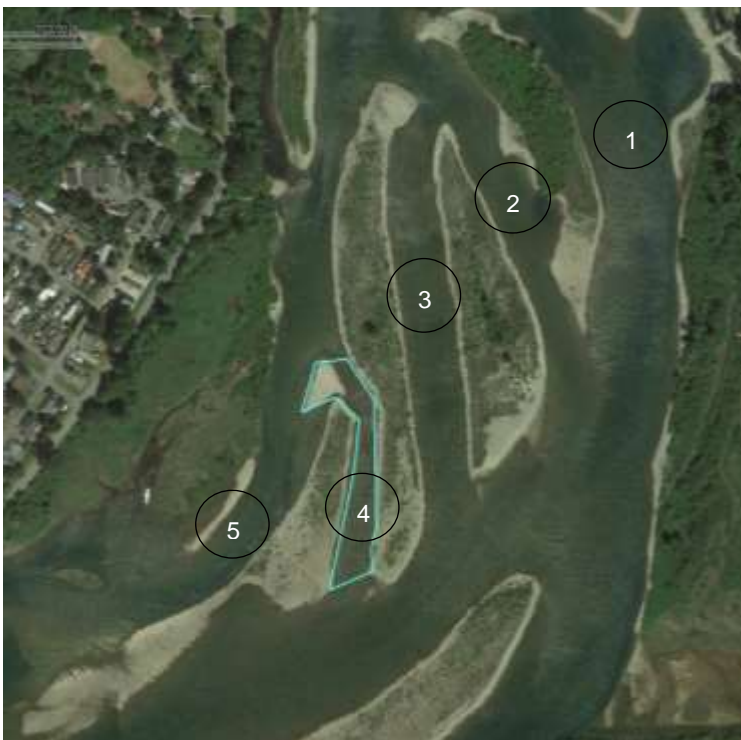
Map 2. Actual area 6,000m 2 shown as a blue line excavated and re-graded to restore flows into Channel 5. (Channels illustrated by circled number)
