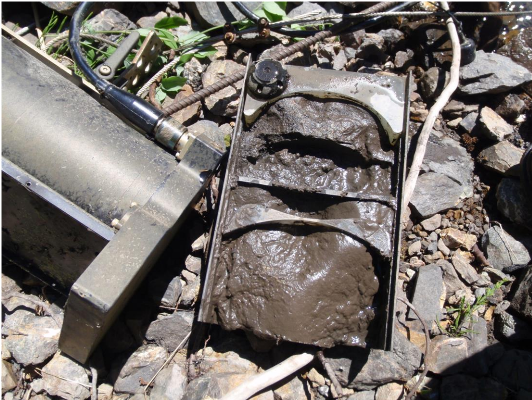
Picture 6. Accumulated silt in DIDSON June, 2010
