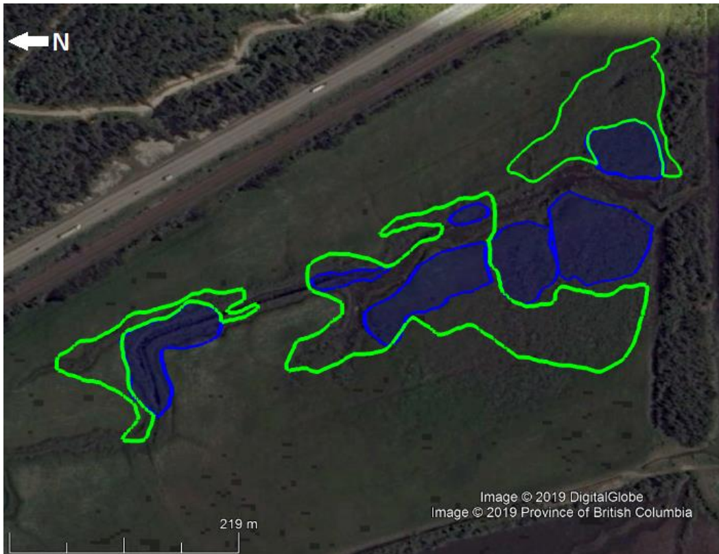
9. Satellite image of works completed on Elk Spike Farm with blue depicting the wetland habitat restored and green depicting where excavated soils were spread.
