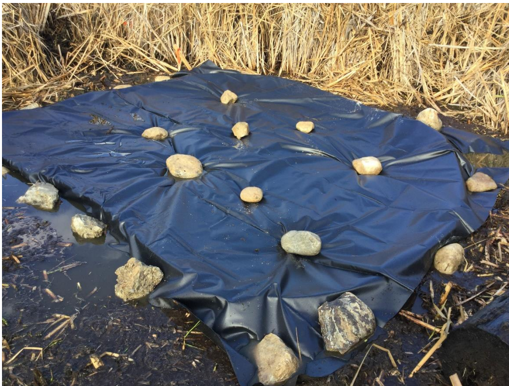
Figure 6. Rocks holding down the benthic barriers at a test plot.
