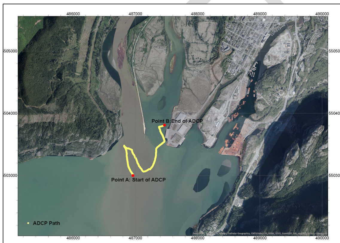
Figure 9 Vessel track for ADCP current measurement on February 16th 2017
