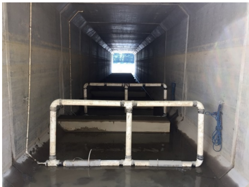
Photo image of acoustic array in Culvert #3 to monitor fish passage between Squamish River and estuary
