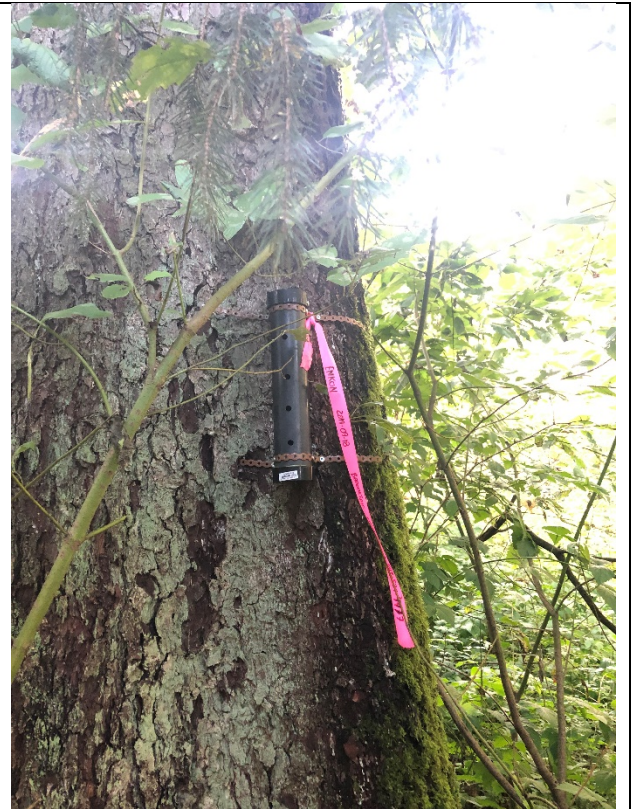
Photograph 11 – Barometric datalogger deployment installed above limits of potential floodplain inundation.
