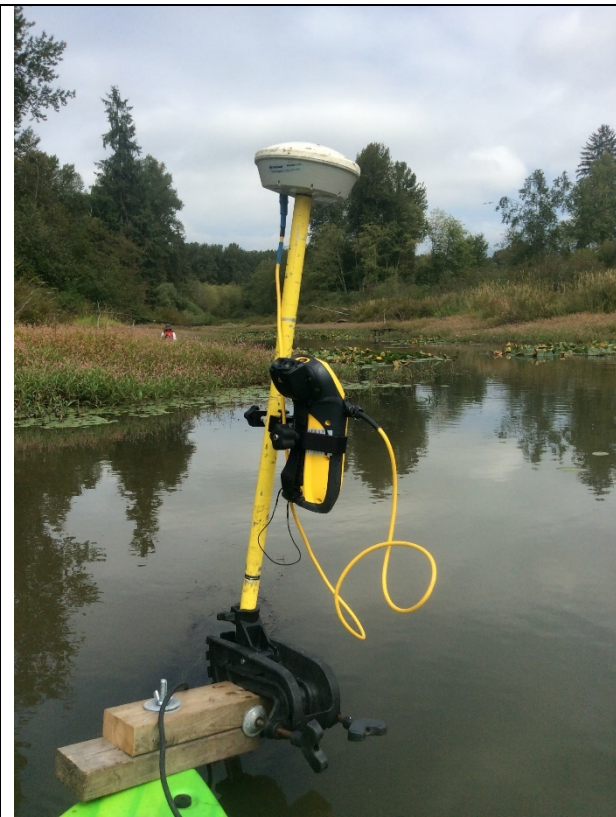
Photograph 8 – Bathymetric survey transducer and GNSS equipment mounted to a kayak at Reeve Slough
