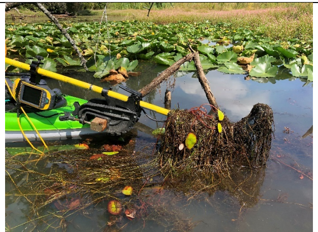
Photograph 9 - Illustration of typical transducer fouling resulting from extensive aquatic weed presence within Reeve Slough.
