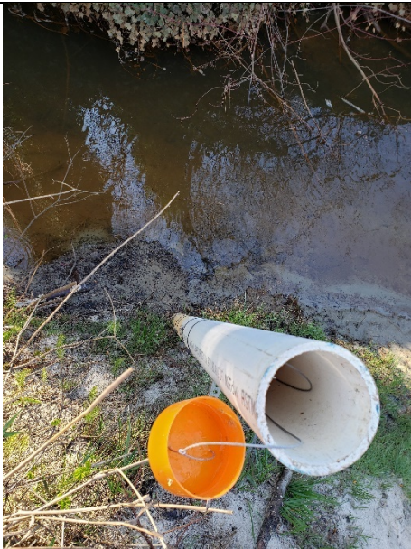
Photograph 12 – Illustration of observed April 2020 conditions at Coquitlam River Levellogger deployment illustrating equipment above low water level.
