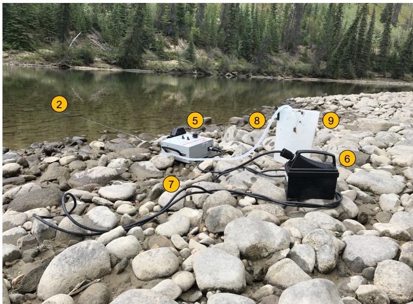
Figure 3.2. The filter apparatus for eDNA sample collection consisted of the peristaltic pump (5), pump battery (6), power cord (7), tubing with funnel adaptor (8), filter assembly (2), and 5L outflow bucket (9).
