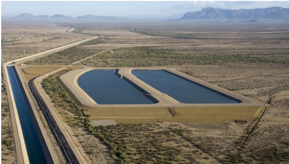
Figure 4: Oblique aerial view of MAR recharge basins (Superstition Mountains) Arizona (USA). Source: Central Arizona Project https://www.cap-az.com .
