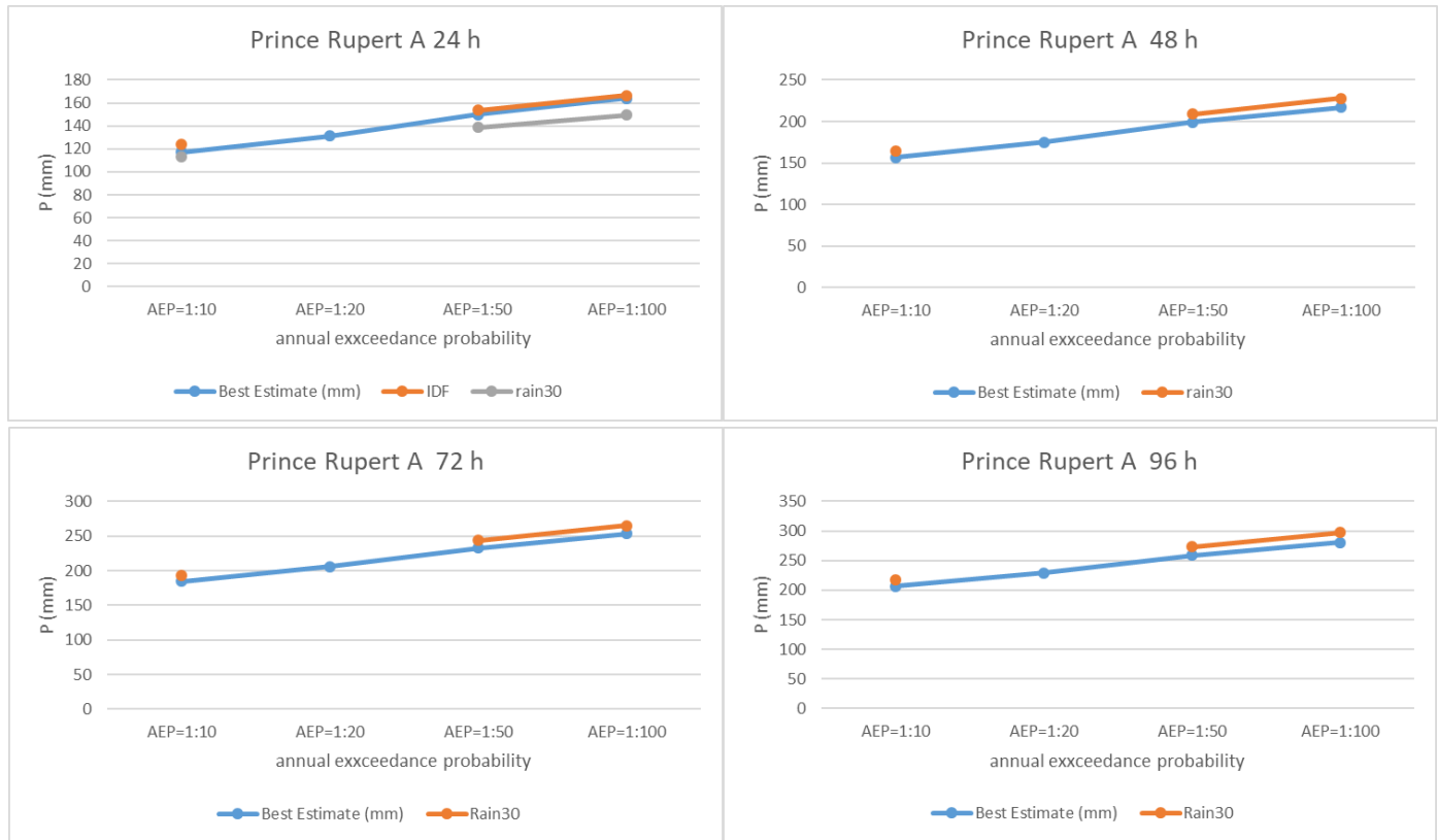
Figure 47: Comparison of point precipitation magnitudes for 1:10, 1:50, and 1:100 AEPs at the four durations of interest for Prince Rupert.
