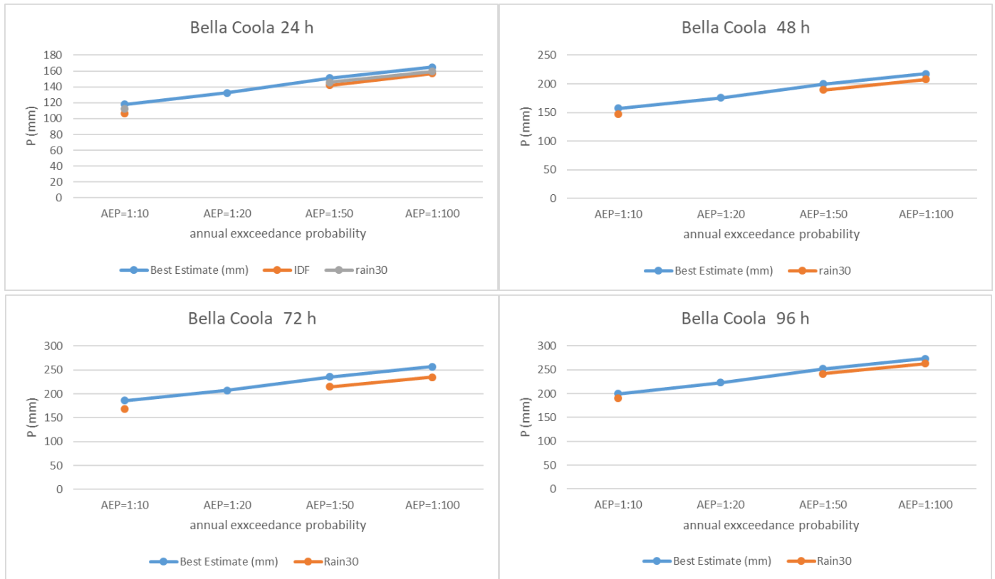
Figure 77: Comparison of point precipitation magnitudes for 1:10, 1:50, and 1:100 AEPs at the four durations of interest at Bella Coola (52.366°N, 126.692°W).
