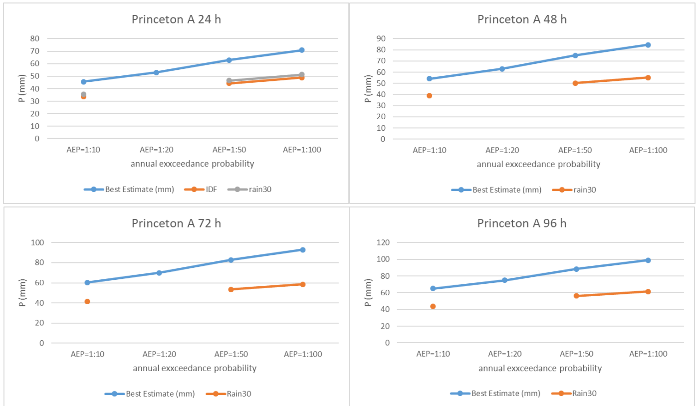
Figure 89: Comparison of point precipitation magnitudes for 1:10, 1:50, and 1:100 AEPs at the four durations of interest at Princeton (49.468°N, 120.514°W).
