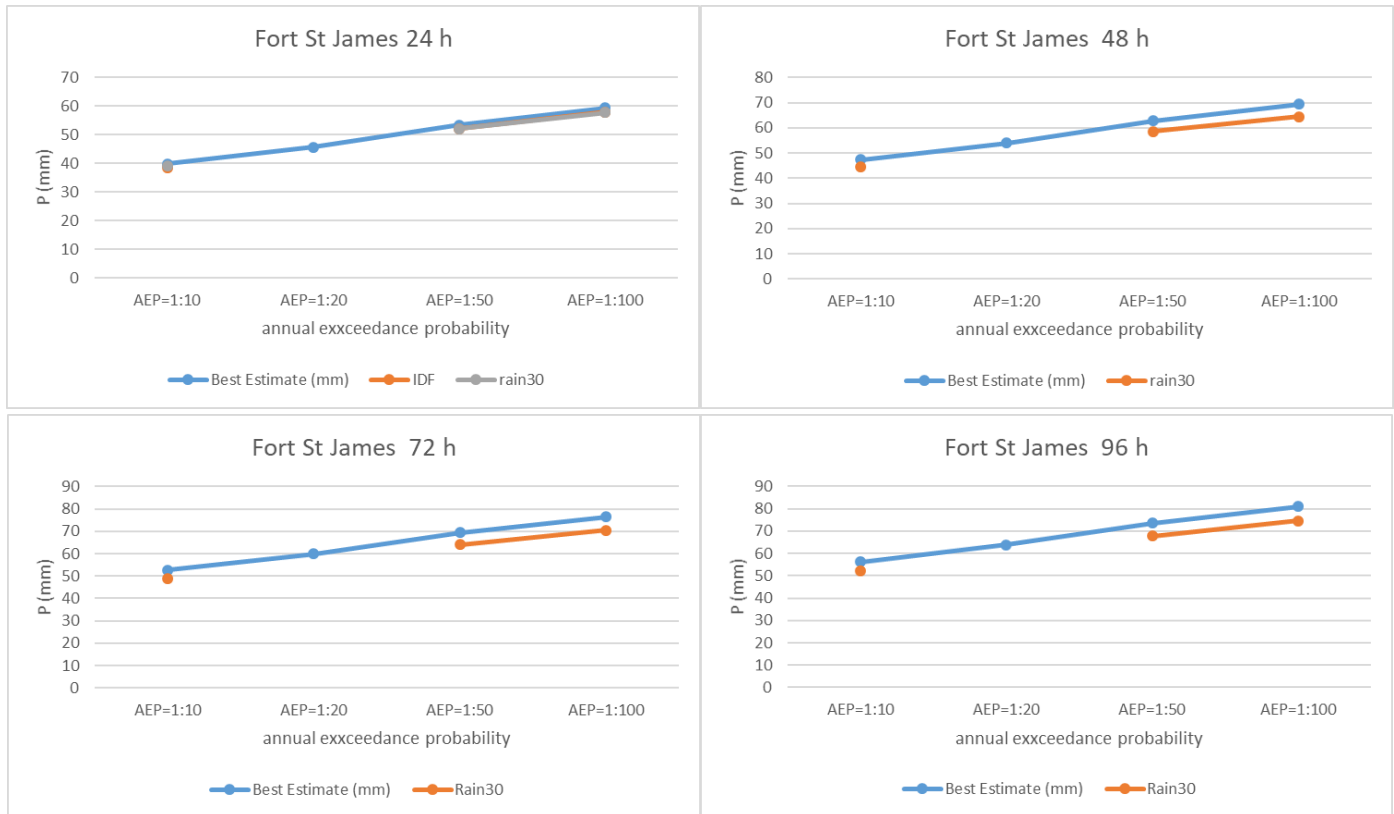
Figure 99: Comparison of point precipitation magnitudes for 1:10, 1:50, and 1:100 AEPs at the four durations of interest at Fort St. James (54.440°N, 124.254°W).
