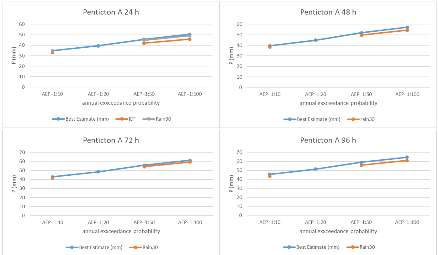
Figure 88: Comparison of point precipitation magnitudes for 1:10, 1:50, and 1:100 AEPs at the four durations of interest at Penticton (49.460°N, 119.603°W).
