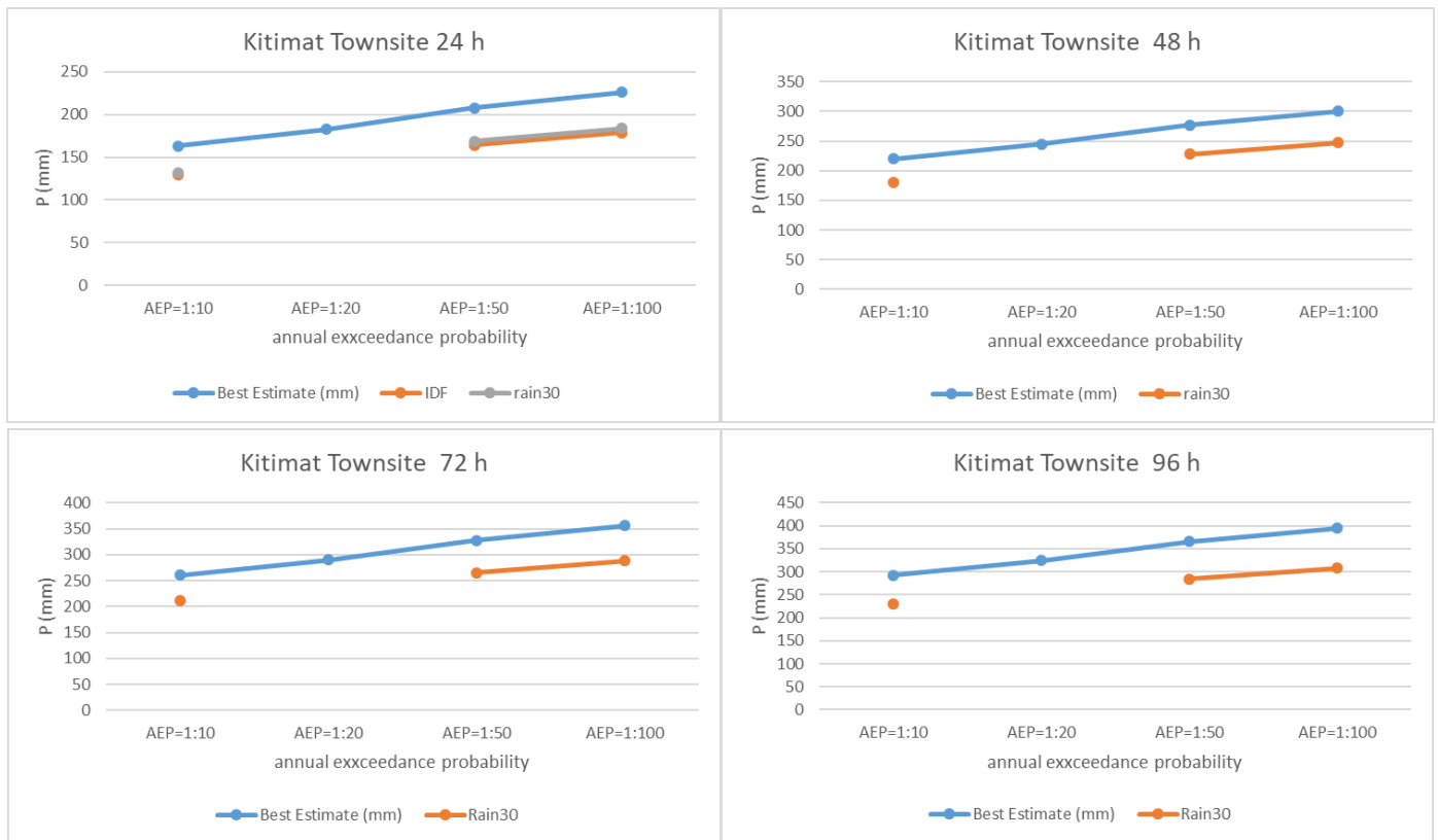
Figure 76: Comparison of point precipitation magnitudes for 1:10, 1:50, and 1:100 AEPs at the four durations of interest at Kitimat Townsite (50.057°N, 128.631°W).
