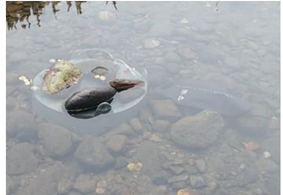
Seepage meter installed under water to measure flux through the stream bed. Photo: J. Wick
