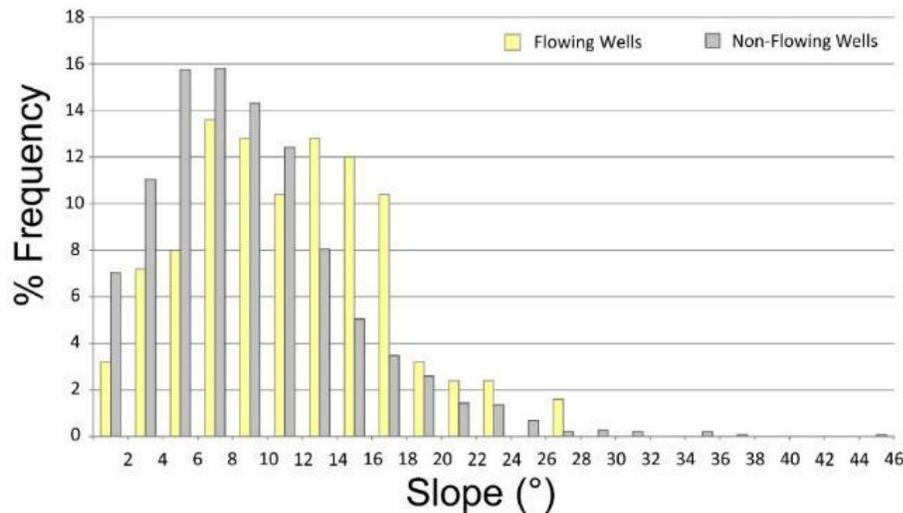
Figure 12: Percent frequency of the occurrence of flowing and non-flowing wells for the slope factor in the Okanagan bedrock context.
