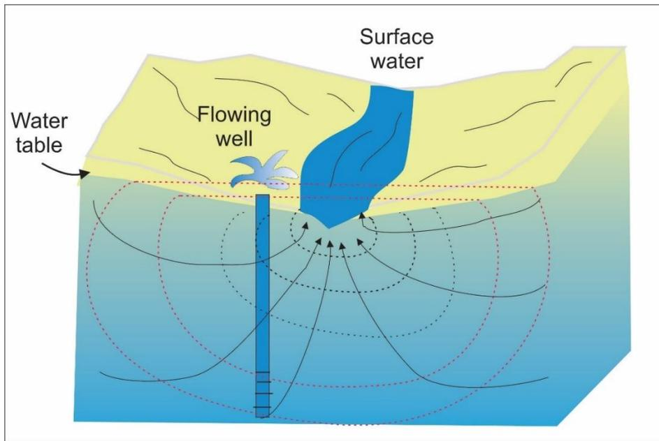
Figure 3: Flowing artesian conditions in topography-controlled unconfined aquifer (modified from Gaber, 2005). The two equipotential lines intersected by the well screen are associated with hydraulic head values above ground surface, as illustrated by the red horizontal dashed lines above the surface. Adapted from B.C. Ministry of Environment, no date).
