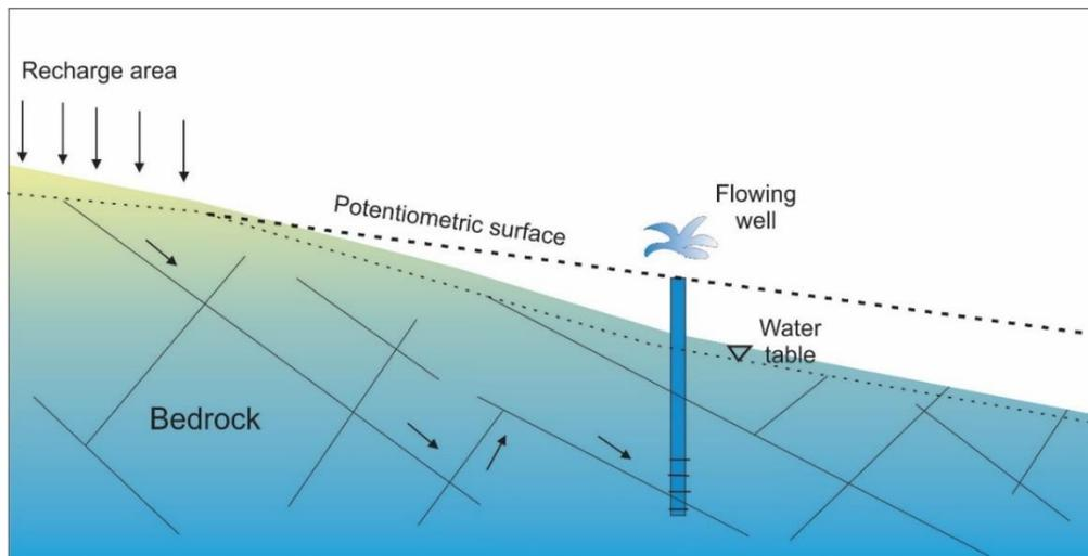
Figure 2: A fractured bedrock aquifer illustrating flow paths along fractures that connect to a recharge area at higher elevation to result in the potentiometric surface above ground surface at the location of the flowing well (modified from Casewell, 1987).
