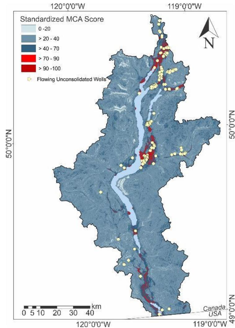
Figure 18: Okanagan unconsolidated MCA maps showing the locations of flowing wells in unconsolidated materials. Red cells indicate where flowing wells are 'more likely than not' to occur and blue cells indicate where non-flowing wells are more likely to occur.
