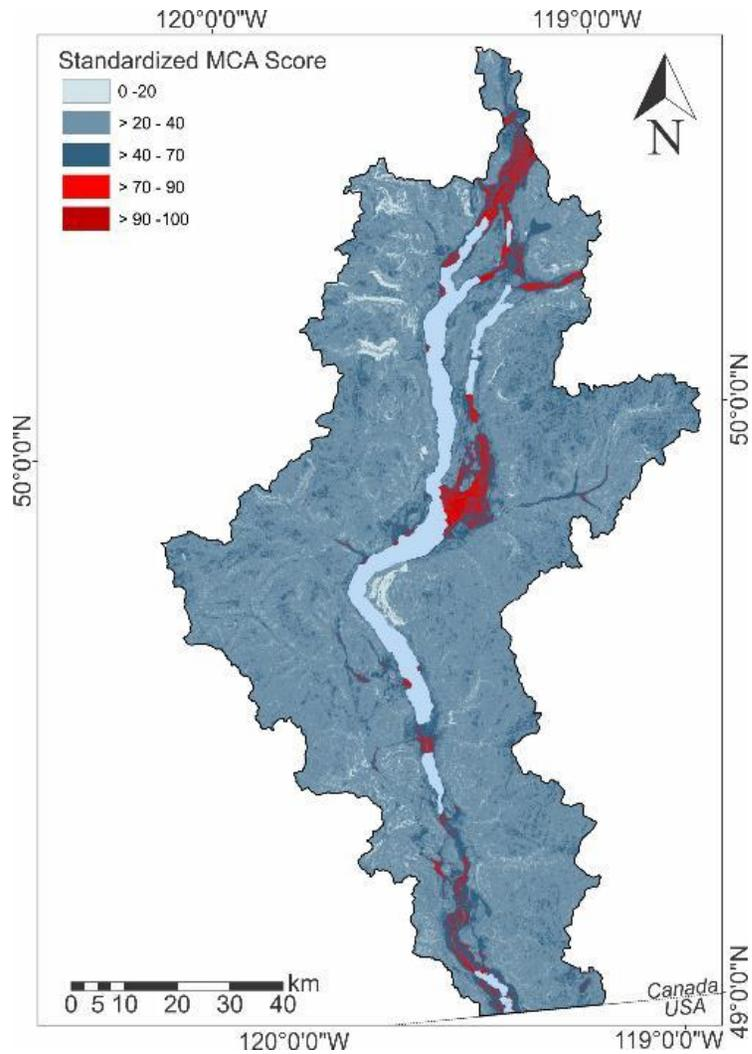
Figure 17: Okanagan unconsolidated MCA map. Red cells indicate where flowing wells are 'more likely than not' to occur and blue cells indicate where non-flowing wells are more likely to occur.
