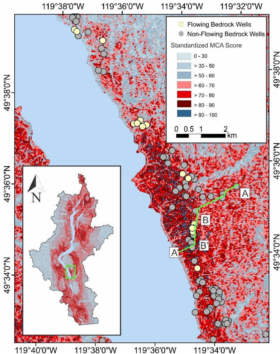
Figure 25: Okanagan bedrock context MCA mapping results in the Naramata region showing flowing and non-flowing bedrock wells. The inset map shows the extent of Naramata (green rectangle). The green line represents the transect for the 2D conceptual model (Figure 26).
