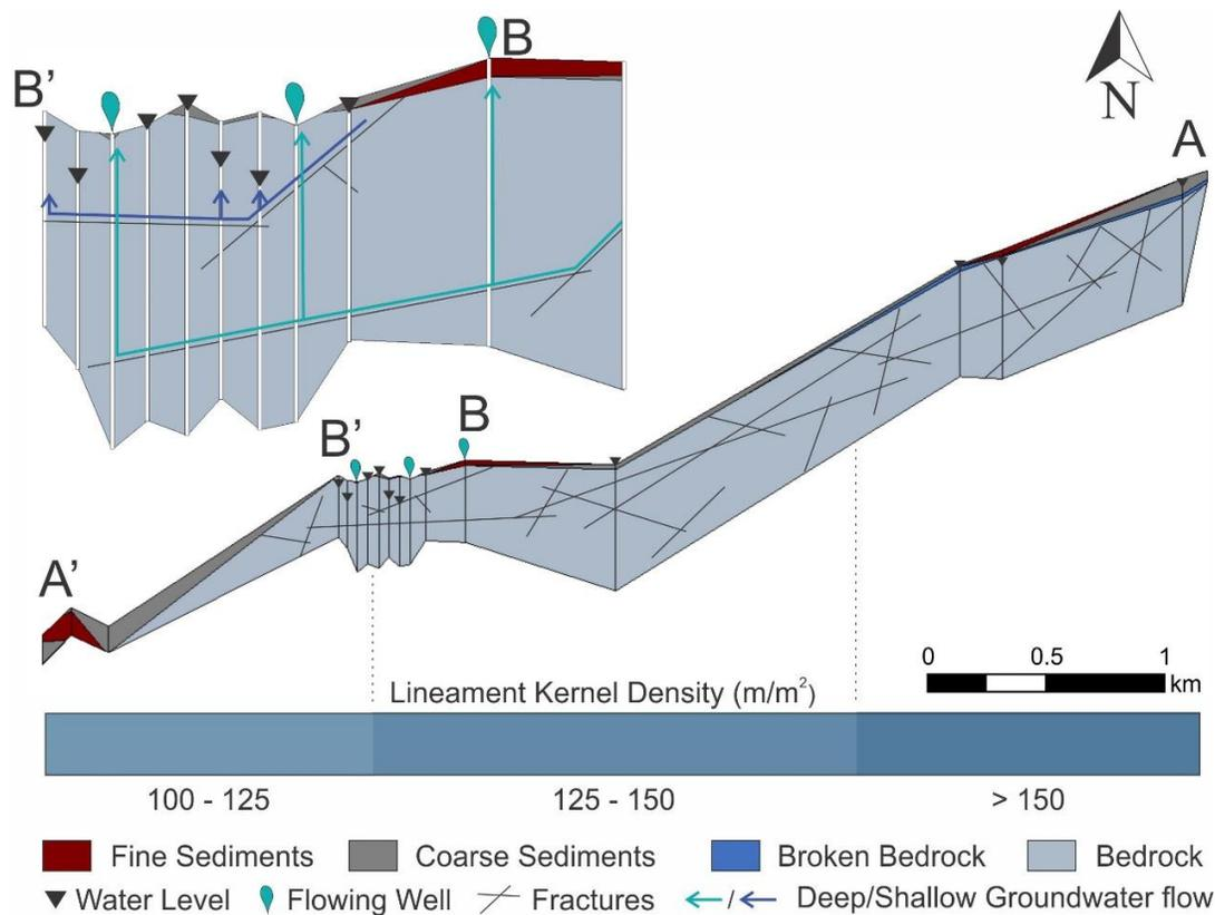
Figure 26: Two-dimensional (2D) conceptual model of flowing bedrock wells in Naramata. Lineament kernel density values determined in Figure B7 are shown along the bottom of the figure. The larger scale inset shows conceptual groundwater flow paths in the fractures which would lead to flowing and non-flowing wells. The model is constrained by ground surface elevation and the depth of the wells (2x vertical exaggeration).
