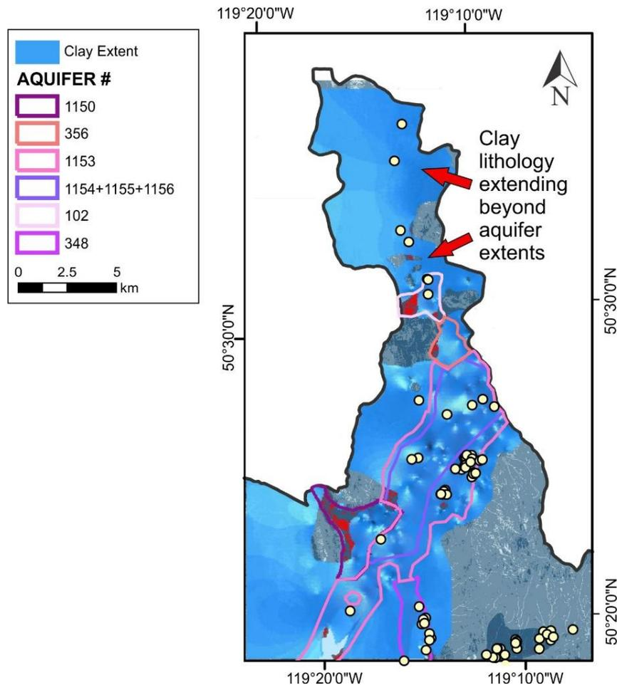
Figure 29: The Leapfrog extent of clay in the Armstrong area with the MCA unconsolidated results showing flowing wells in unconsolidated materials and the outlines of the mapped confined aquifers superimposed. Red arrows indicate the extent of the clay unit beyond the confined aquifers.
