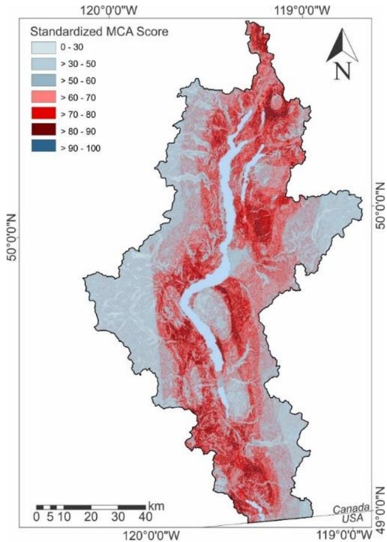
Figure 14: Okanagan bedrock MCA map. Red cells indicate where flowing wells are 'more likely than not' to occur and blue cells indicate where non-flowing wells are more likely to occur.
