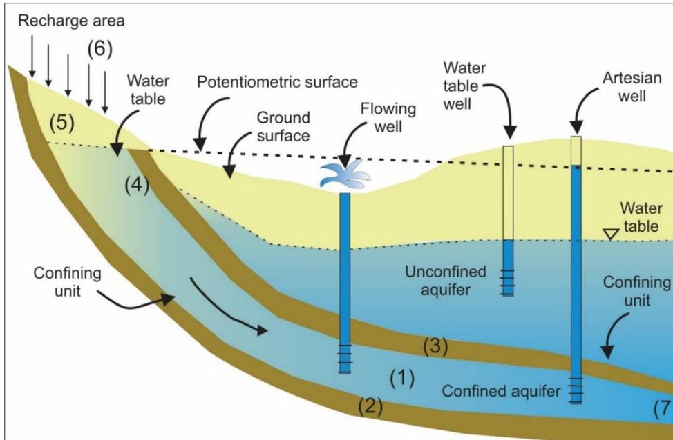
Figure 1: Geologically-controlled artesian conditions which result in flowing wells due to the potentiometric surface of the confined aquifer above ground surface at the location of the flowing well (modified from Todd, 1959). Numbers in brackets relate to the list above.
