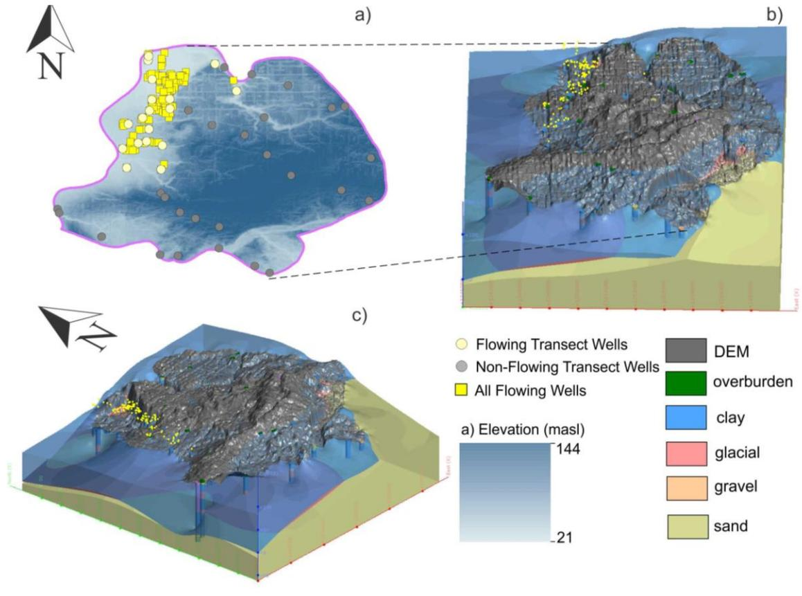
Figure 32: a) DEM of Aquifer 33 with the flowing and non-flowing wells used in the transects (circles) and all flowing wells in the aquifer (squares). b) Leapfrog Geo Model for Aquifer 33 DEM overlay c) Leapfrog model for Aquifer 33 re-oriented.
