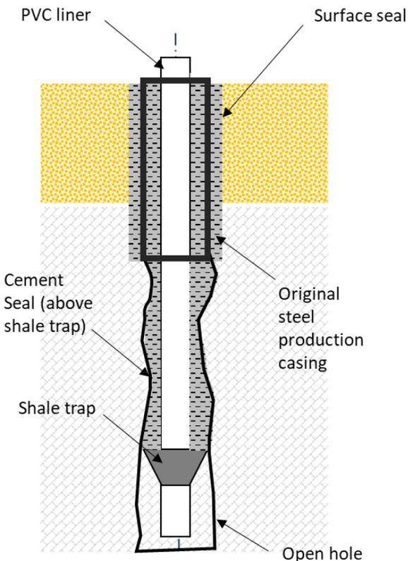
Figure 33: Schematic of a shale trap installed in a bedrock well.
