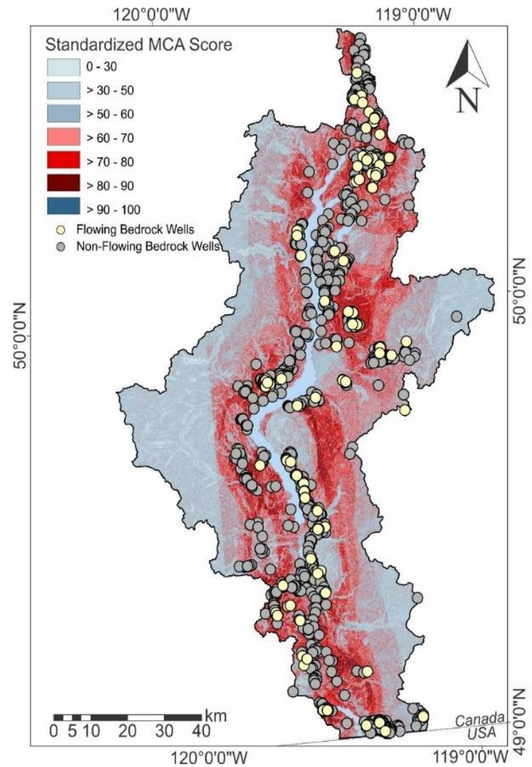
Figure 15: Okanagan bedrock MCA map showing the locations of flowing bedrock wells. Red cells indicate where flowing wells are 'more likely than not' to occur and blue cells indicate where non-flowing wells are more likely to occur.
