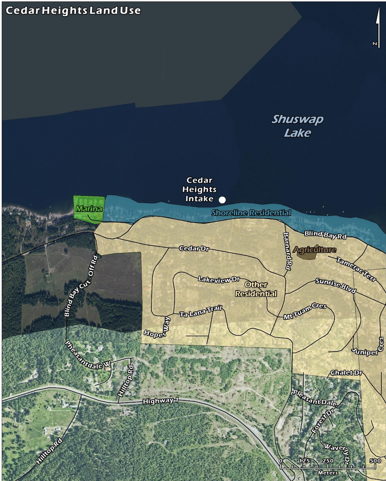
Figure 3.1: Potential hazards to water quality in the vicinity of the Cedar Heights intake. Similar land uses are colour coded.
