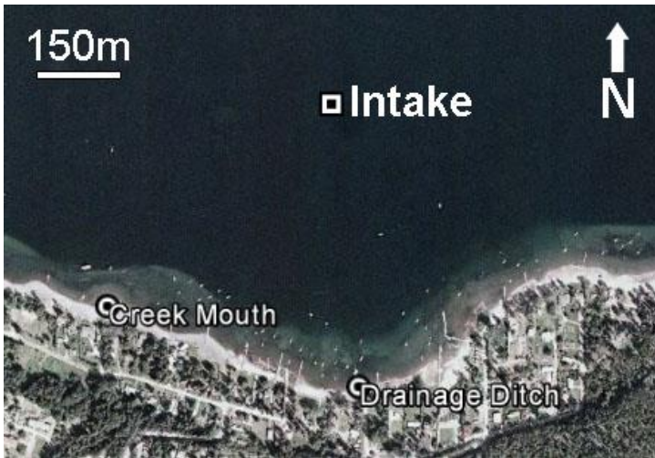
Figure 2.4.1: Major stormwater discharge points near the Sorrento water intake
