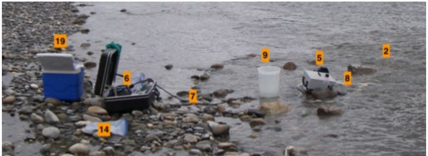
Figure 4: Instream filtering apparatus for eDNA sample collection consisted of the filter assembly (2), peristaltic pump (5), pump battery (6), power cord (7), tubing with funnel adaptor (8), graduated outflow bucket (9), clean sample bag (14), and cooler (19).
