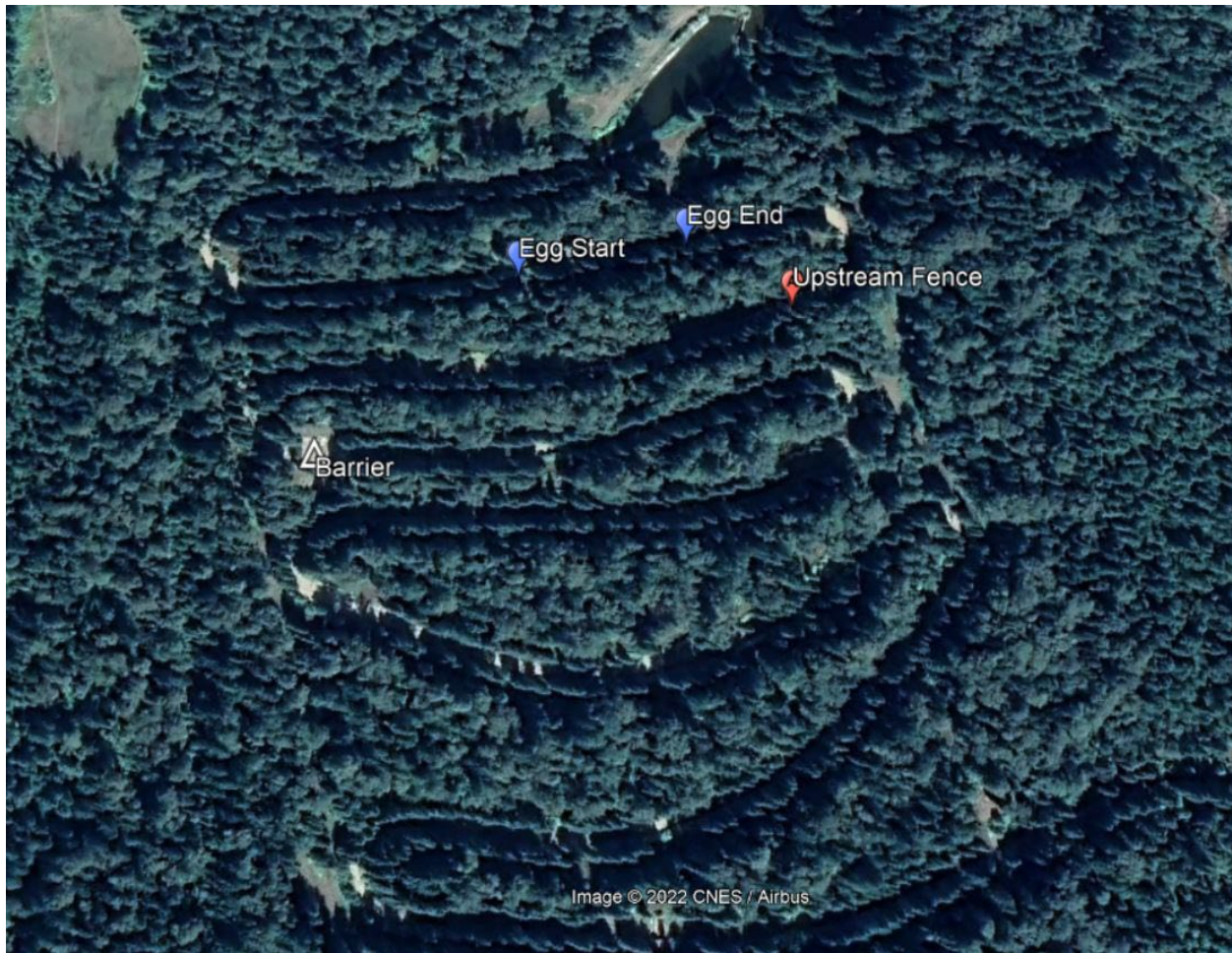
Figure 2. Aerial view of Meadow Creek Spawning Channel showing location of the fish barrier in 2021. Water flow proceeds from the settling pond at the top of the photo towards the bottom. The spawning channel downstream of the barrier was surrounded with electric fencing to protect the low escapement of adult Kokanee from bear predation in the channel. The approximate start and end of buried eyed eggs is marked upstream of the barrier as well as the proposed location for a counting fence for fry from the eyed eggs. (Figure by A. Bendis, pers. comm.)
