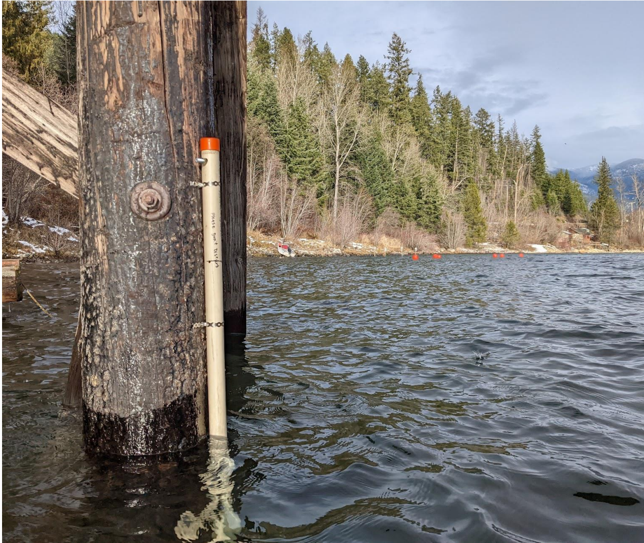
Figure 13: Photo of water level logger measuring lake stage at restoration site. Photo credit: Cameron Spooner.
