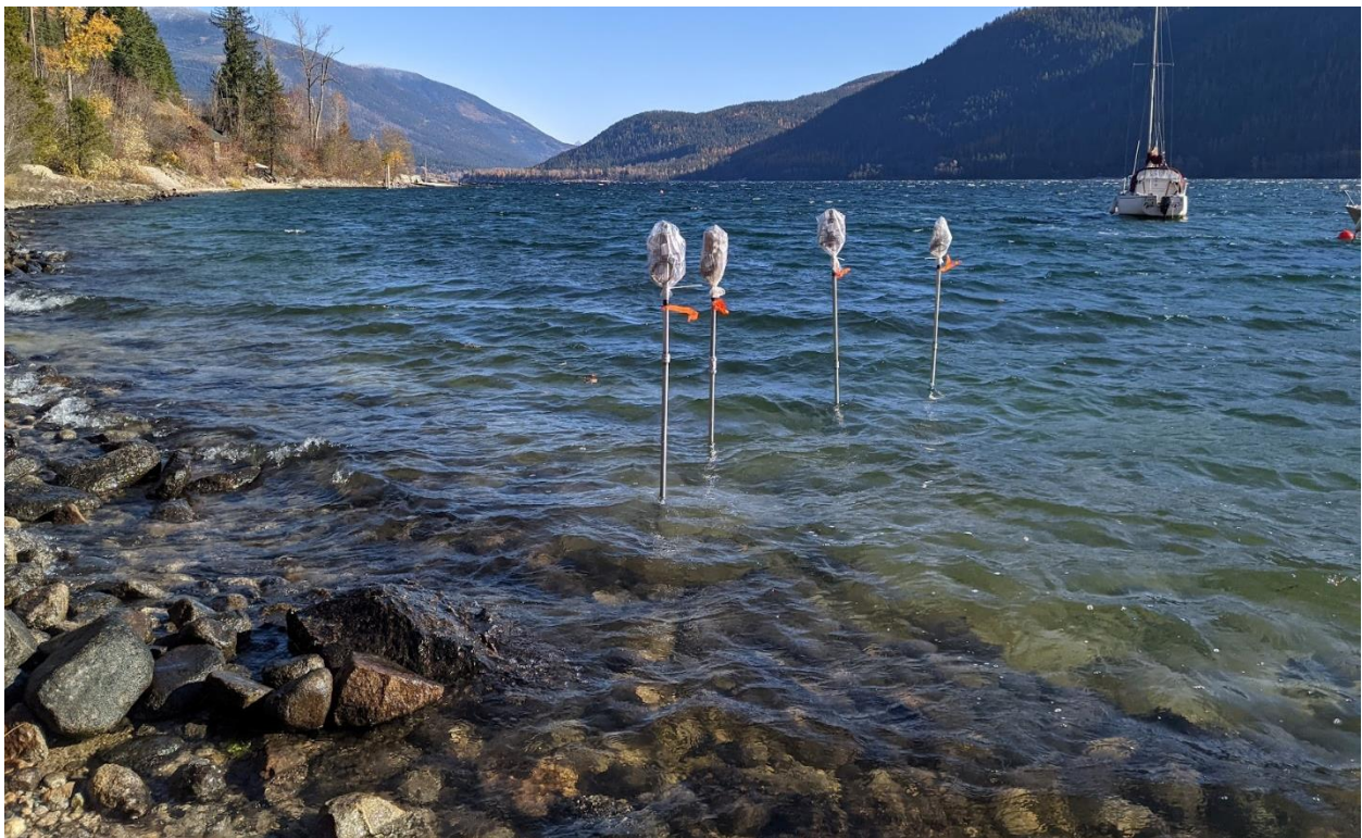
Figure 12: Photo of vertical sediment temperature profiling probes installed at McDonald's Landing restoration site. Photo credit: Cameron Spooner.
