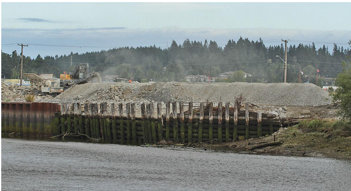
Figure 8- Rock crusher generating windrow piles of crushed concrete.
