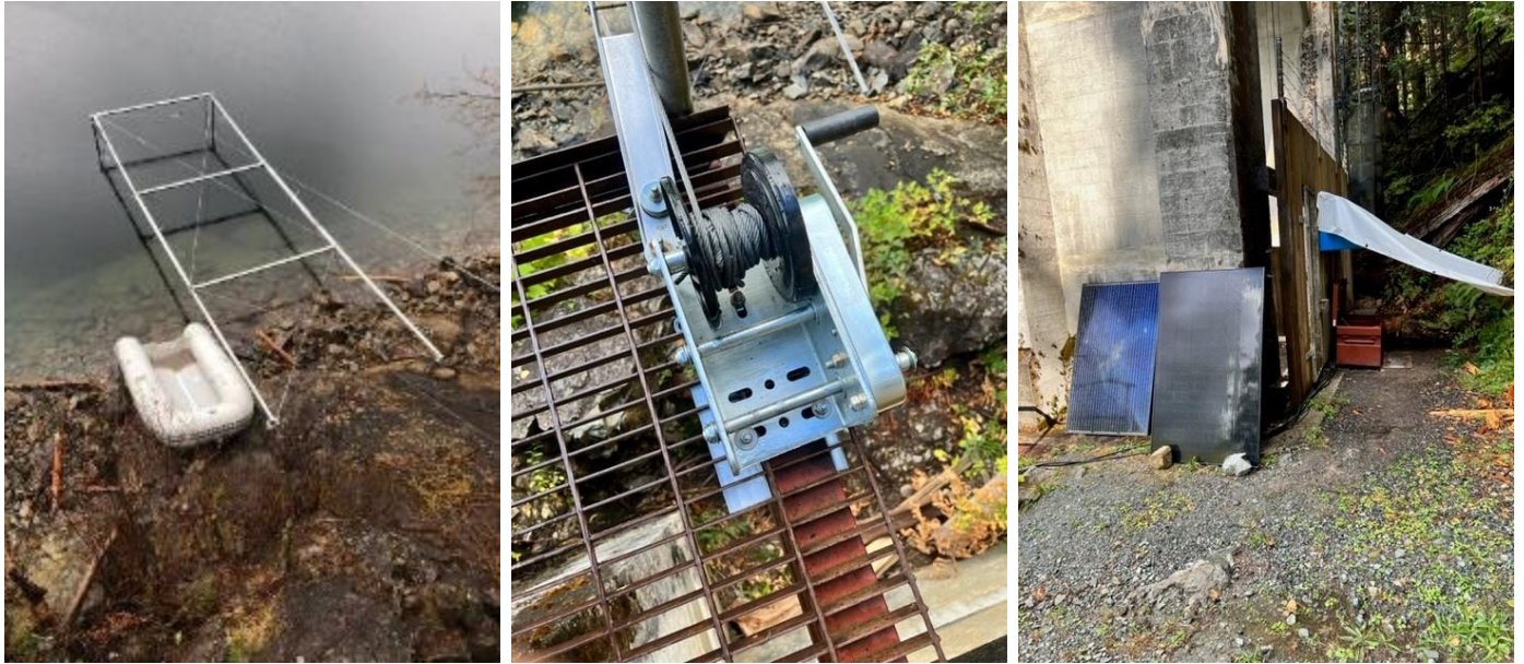
Figure 3.2 Transducer deployment frame (left panel), automatic brake trailer winch (centre panel) used to lower and lift the transducer deployment frame to optimally cover the Tunnel entrance and keep the transducers immersed, and complete set-up with solar panels.
