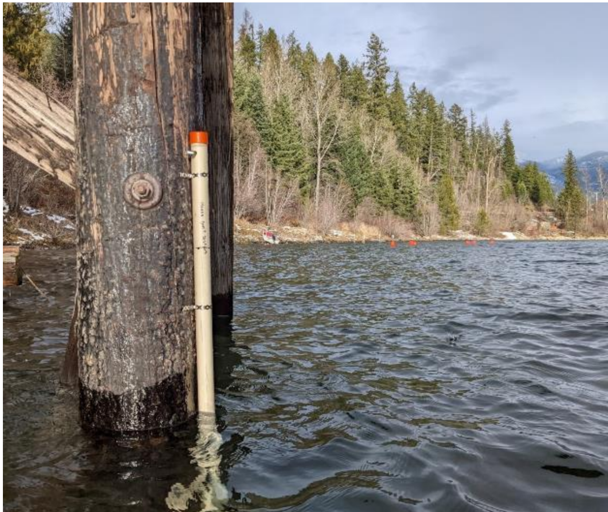
Figure 11: Photo of water level logger measuring lake stage at restoration site. Photo credit: Cameron Spooner.
