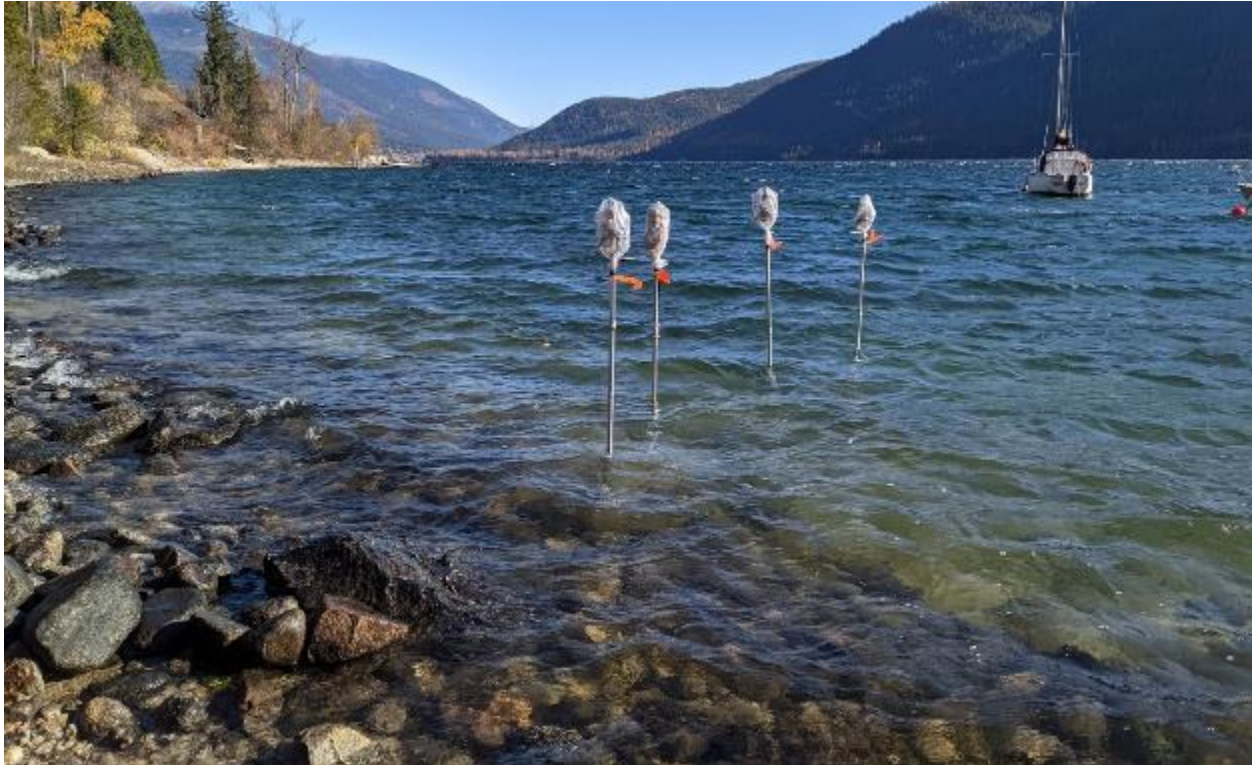
Figure 10: Photo of vertical sediment temperature profiling probes installed at McDonald's Landing restoration site. Photo credit: Cameron Spooner.
