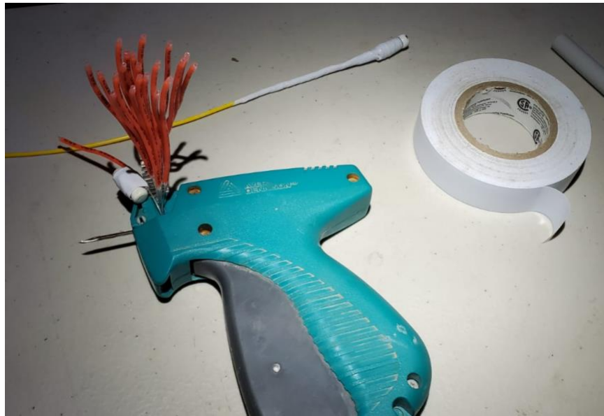
Figure 12. A pair of synchronized Star ODDI DST Nano-T loggers prepared for internal and external application.
