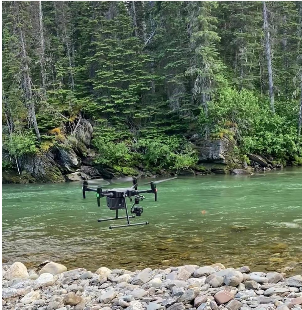
Figure 4. DJI Matrice 200 V2 quadcopter drone equipped with a Zenmuse XT2 RGB+FLIR camera on a downward facing (nadir) gimbal mount.
