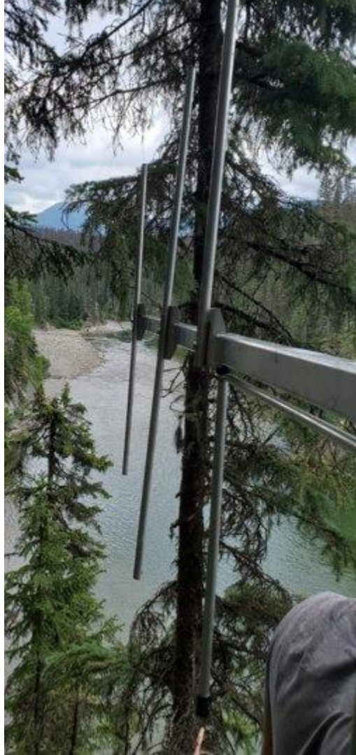
Figure 14. Radio receivers were set up at vantage points along each study reach.
