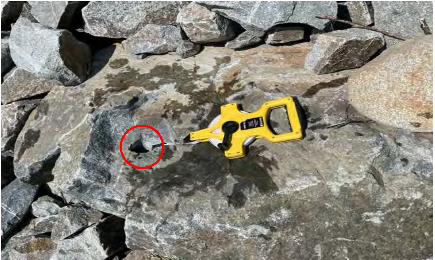
Figure 45. Benchmark. Used same benchmark feature for all structures at NNSC. (Hole in rock)
