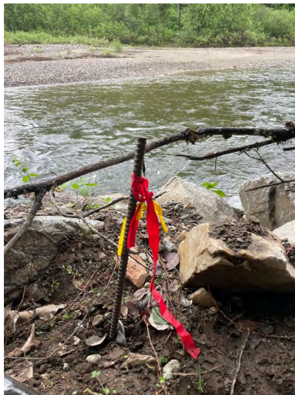
Figure 27. Benchmark for downstream arm of fourth W and fourth triangle (last structure).
