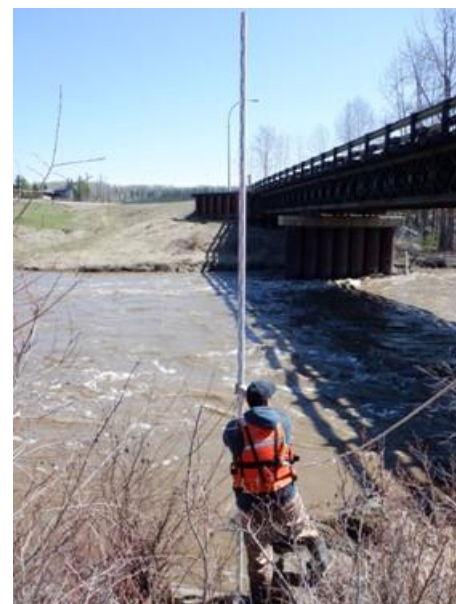
High flow water level survey, Doig River. Photo: R. Rolick.
