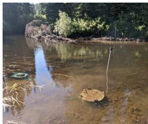
In-stream piezometer and seepage meter Photo: J. Wick
