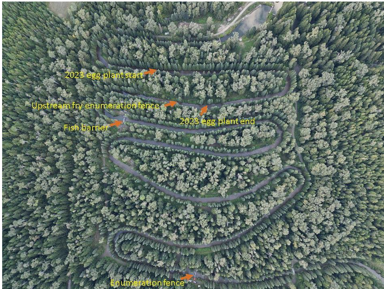
Figure 3. Aerial view of Meadow Creek Spawning Channel showing location of the fish barrier. Water flow proceeds from the settling pond at the top of the photo towards the bottom. The spawning channel downstream of the barrier was surrounded with electric fencing to protect the low escapement of adult kokanee from bear predation in the channel. The approximate location of the eyed egg plants is between “2023 egg plant start” and “2023 egg plant end”. The Upstream Fence is the enumeration location for the fry of upstream plants, and the lower enumeration fence is for counting returning spawning kokanee in fall and naturally spawned fry in spring.
