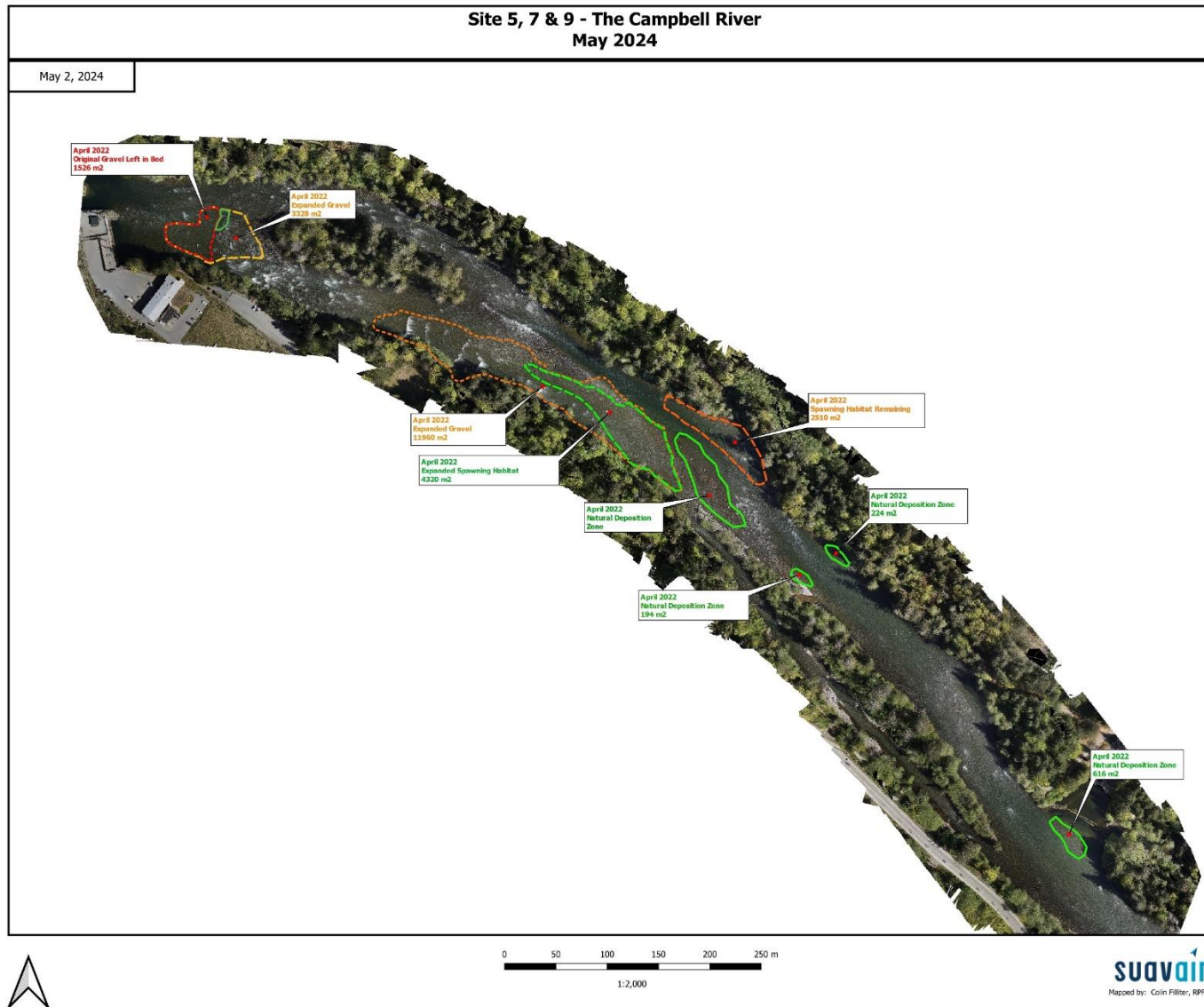
Figure 2: Orthomosaic of the upper reach of the Lower Campbell River from the powerhouse to the Elk Falls water intake with details of gravel restoration projects and depositional zones that have suitable spawning habitat.
