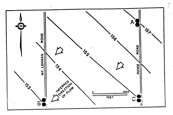
Figure 5. Water table elevation contours, in feet above sea level and inferred direction of flow between piezometer sites, June 1988.
