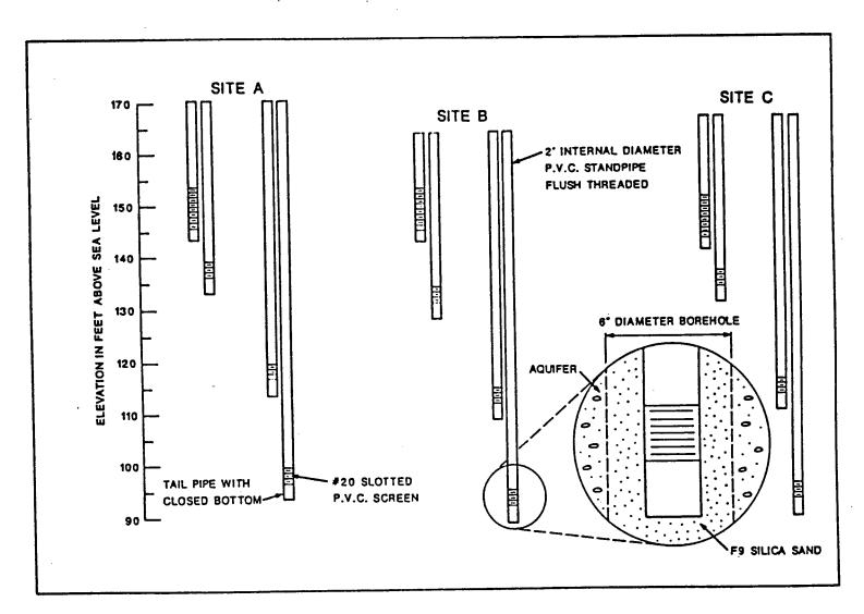
Figure 4. Piezometer settings and construction details.
