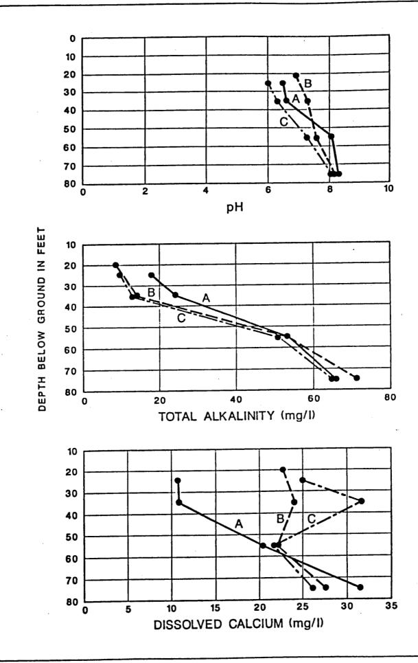
Figure 7. Variations of pH, total alkalinity and dissolved calcium with depth.
