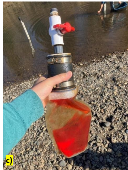
Figure 15: Seepage metre system design (a), field installation (b), and a closer look of the collection bag (c). The food colour was initially added to the water to test for potential leakage and to ensure the free flow of water in the system.
