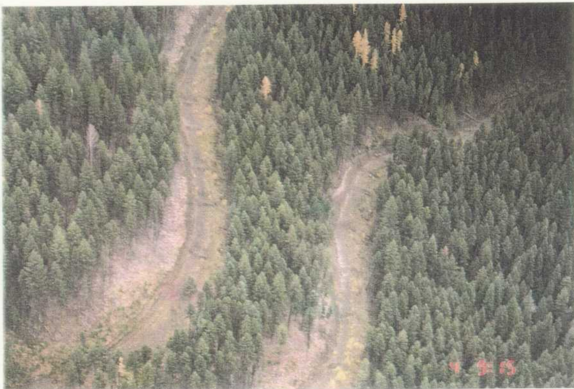
Photo 6. Upper Ferry Creek, Road FE4, Section 1. Semi-permanent deactivation. Frequent water bars.
