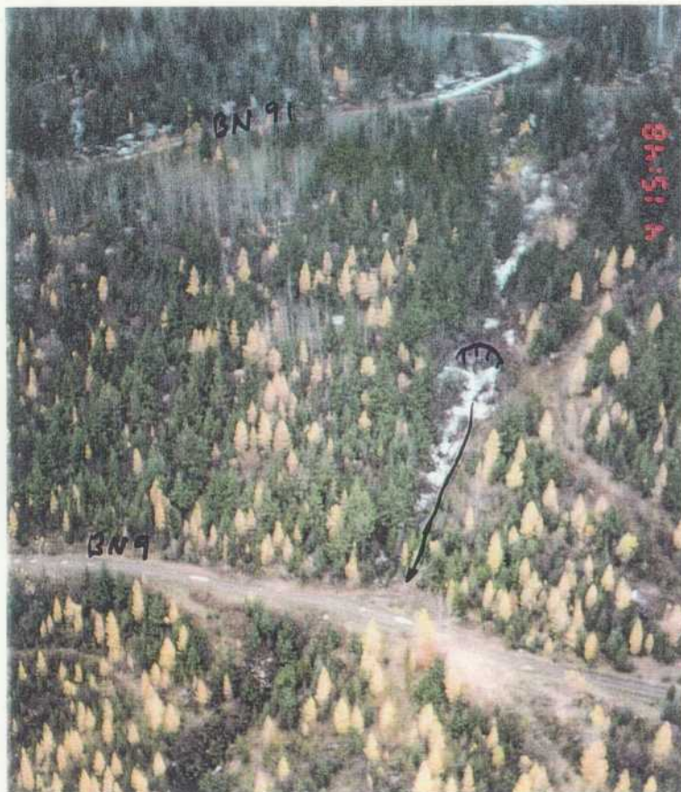
Photo 17. BN9. Road alignments on moderately steep (30 to 50%) slopes. Little sediment movement to perennial streams.
