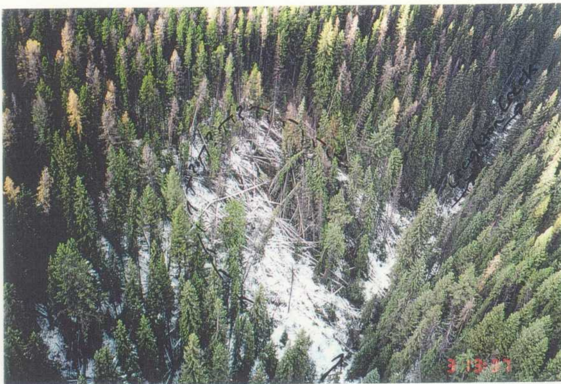
Photo 23. S50. Earth slump ~170m wide, adjacent to Creighton Creek.
