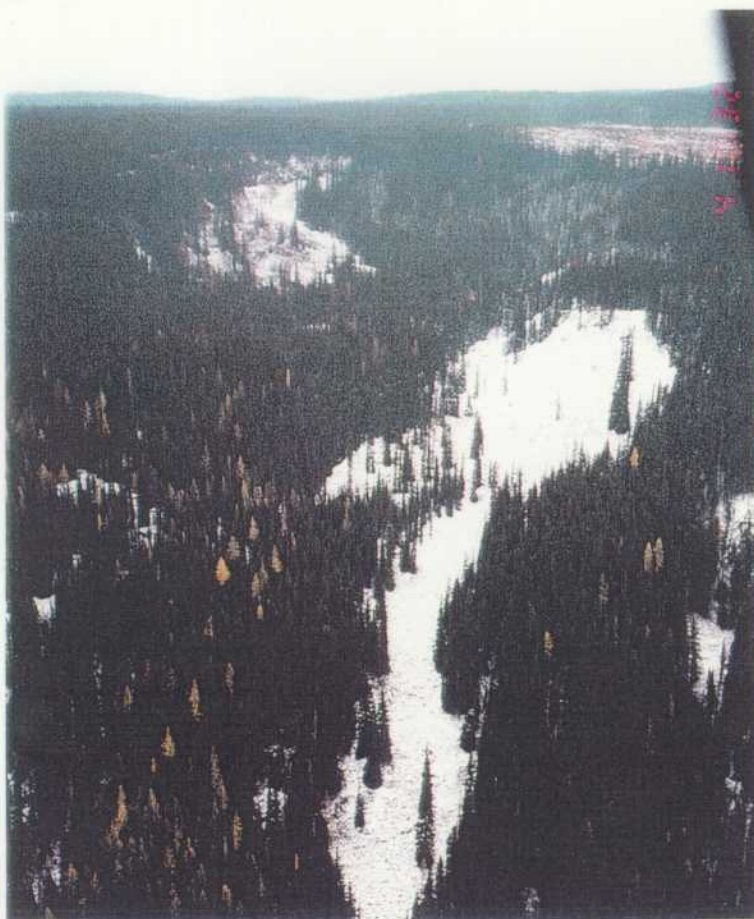
Photo 23. S50. Earth slump ~170m wide, adjacent to Creighton Creek.
