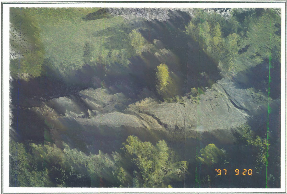
SITE R4B. Aerial view of the mouth of the Black Creek fan. Note the aggradation of gravel. This material has eroded from the fan immediately upstream, and from the placer mining operation about 1 kilometre upstream.
