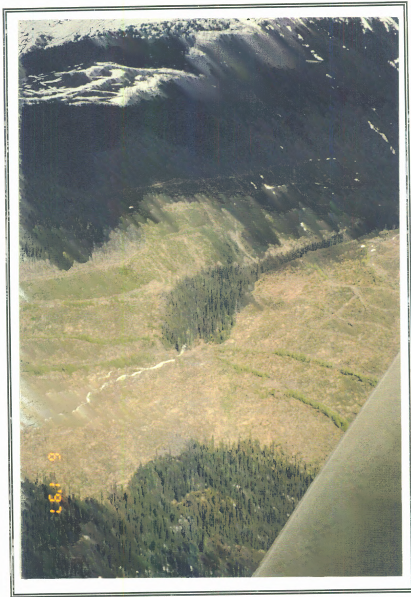
PHOTO MCKAY5. Extensive development on unstable terrain in Pegasus Creek. Multiple landslides into channel and riparian harvesting on the alluvial fan [ Site McKay8 ].
