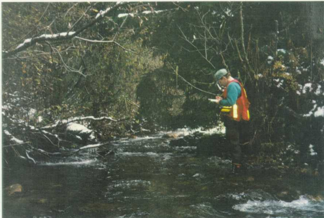
Upstream view of Reach 8, Monashee Creek has minimal pool area, therefore, indicating an aggrading channel.
