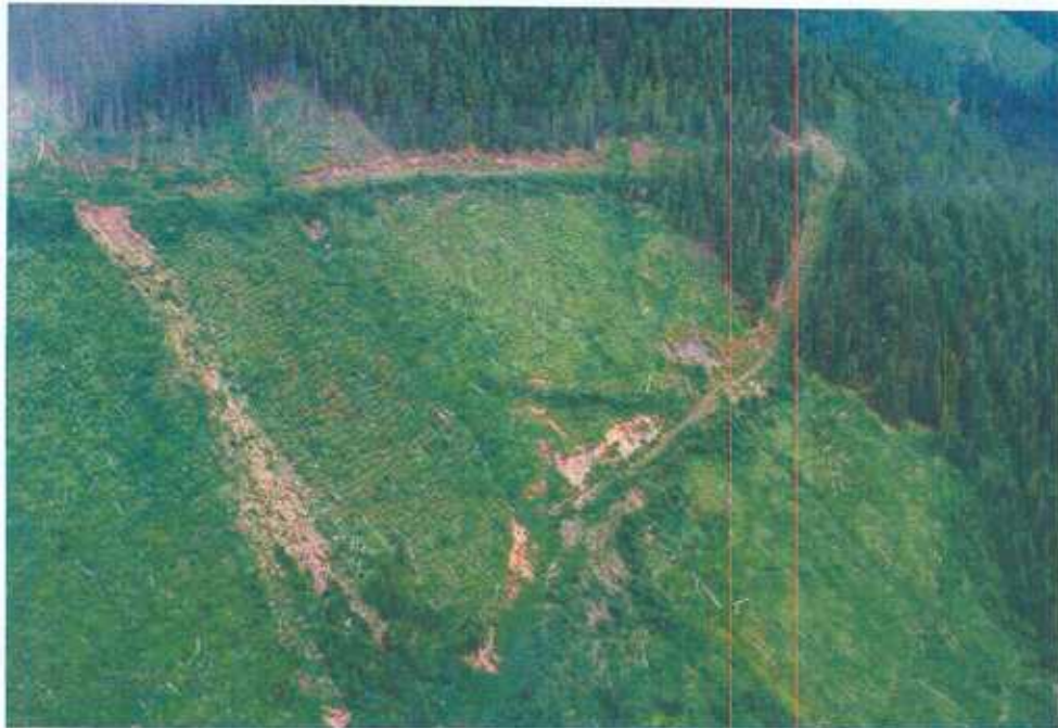
Photo 45: Lempriere watershed – Unnumbered slide initiated at Road 1303.02. Located within opening 18, polygon 167.
